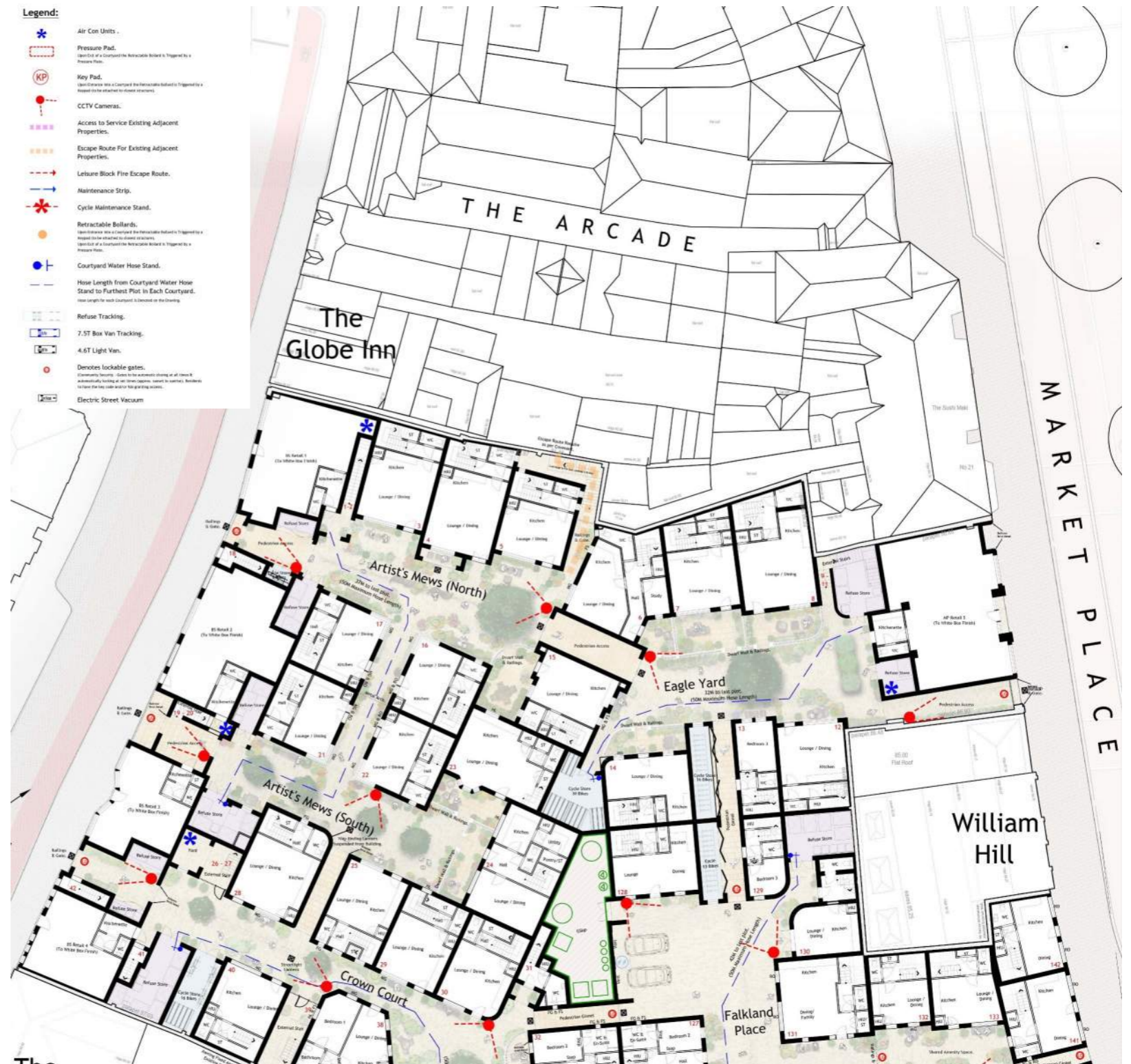
Figure 6.79: Proposed Fire Escape route from The Globe Inn boundary through the proposed development (Extract of the Servicing & Security Plan 19401/1036).
