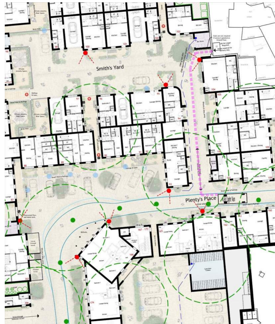
Figure 6.83: Proposed Servicing route to the r/o the Catherine Wheel PH through the proposed development (Extract of the Servicing & Security Plan 19401/1036).
