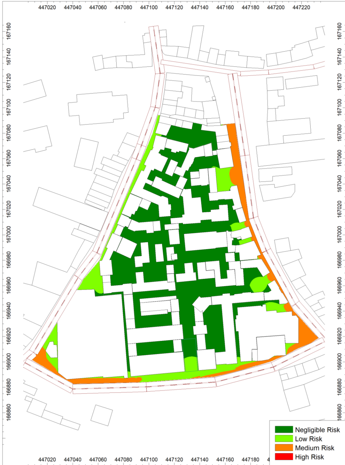
Figure 5.1: Initial daytime site noise risk assessment ( L_{Aeq,1\text{hour}} road traffic noise contours predicted at 4.5 metres above ground level)
