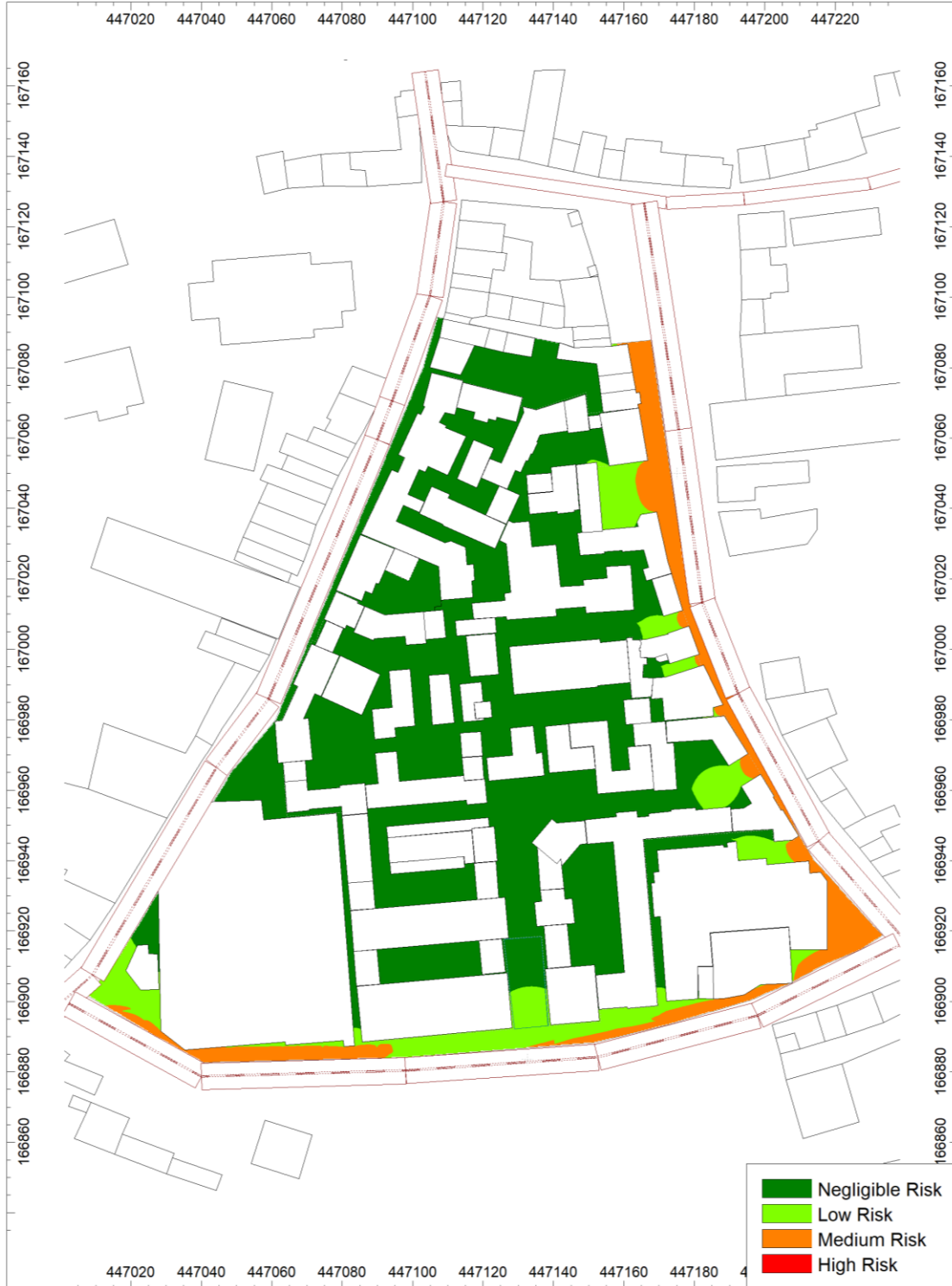
Figure 5.2: Initial night-time site noise risk assessment ( L_{Aeq,8hour} road traffic noise contours predicted at 4.5 metres above ground level)
