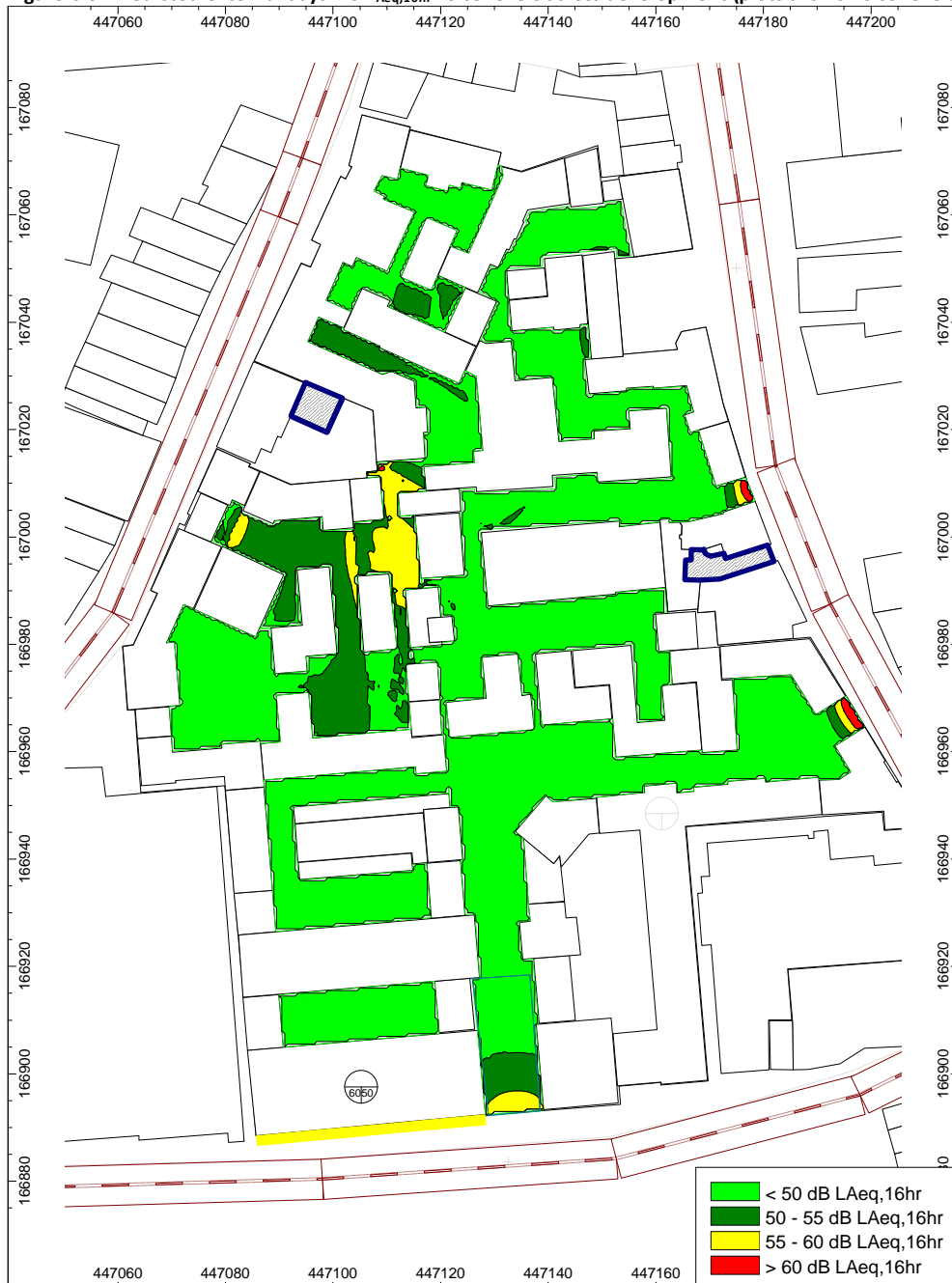
Figure 6.9: Predicted external daytime L_{Aeq,16hr} noise levels across development (plots shows noise levels at 3 rd floor level)
